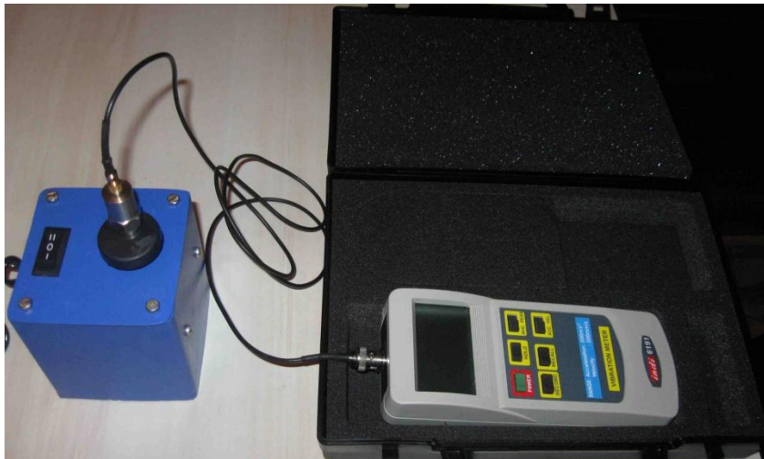
Displacement, Velocity & Acceleration Measurement Set Up (SAP - 27)
