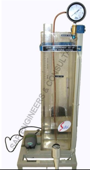
AIR PURGE BUBBLER SYSTEM FOR LEVEL MEASUREMENT (SAP –47)
